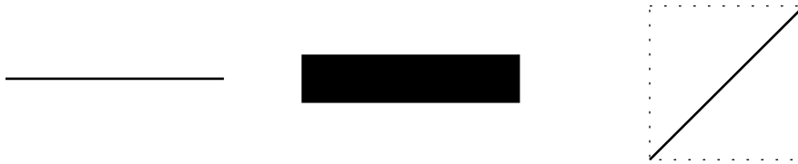
Figure 5. This figure illustrates the effect of stroke-width and rotation on the actual bounding box of a line. These three lines are all of the same length. The left line is stroked with a .5 point pen and has a rotation of 0^\circ . The middle line is stroked with a 20 point pen and has a rotation of 0^\circ . The right line is stroked with a .5 point pen and has a rotation of 45^\circ . Its bounding box is shown as a dashed square
