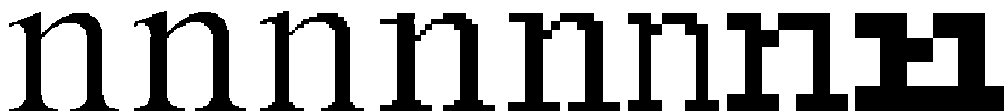
Figure 6. A Times n at various type sizes from 72 pt at 300 dpi down to 9 pt at 72 dpi, showing dynamic regularisation of the stroke thickness and of different serifs
