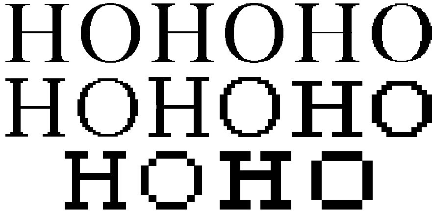
Figure 4. Times HO at type sizes from 72 pt at 300 dpi down to 9 pt at 72 dpi, showing regularisation of the thicknesses of stroke and discrete dropping of reference-line overlaps
