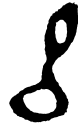
Figure 13. Garamond letter 'g' in metal type. Note the distortions caused by the inking process and by worn type
