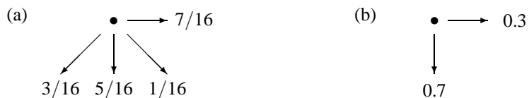
Figure 1. Two examples of diffusion weights. (a) Original diffusion weights proposed by Floyd and Steinberg; (b) Example with two weights
